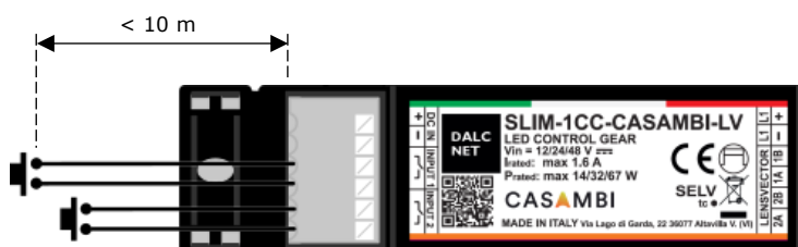
Figure 3: Local Command connection diagram for Short Distances
