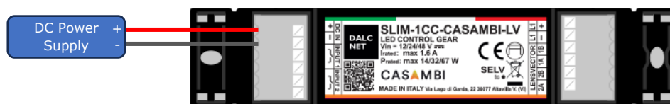
Figure 5: Power Supply Connection Diagram
